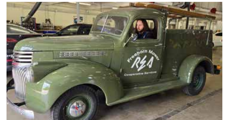
Freeborn Mower Electric Cooperative's 1946 Chevrolet truck had its gas-powered engine replaced with an electric-powered engine.
